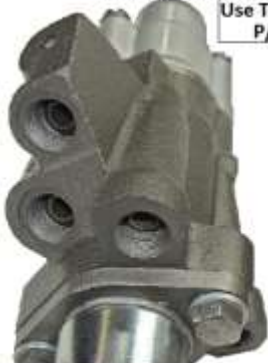
Early Power P/S Control Valves had (3) Large Ports and (1) Small Port.
